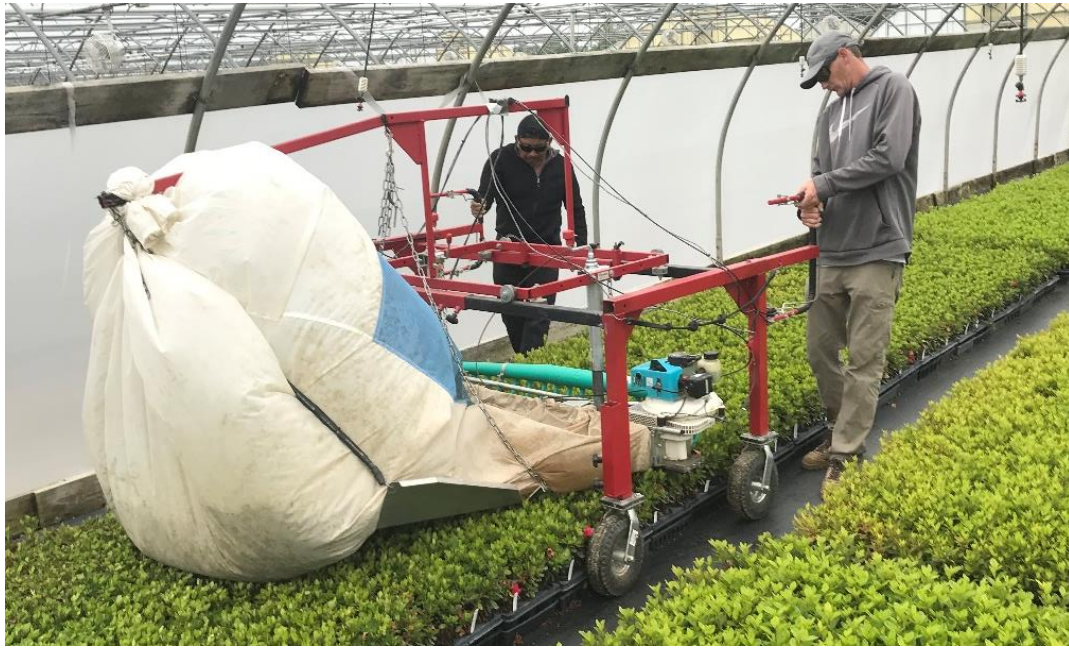
Figure 26. Gas powered sickle bar pruning machine with blower and bag attachment for uniform pruning and debris collection.
