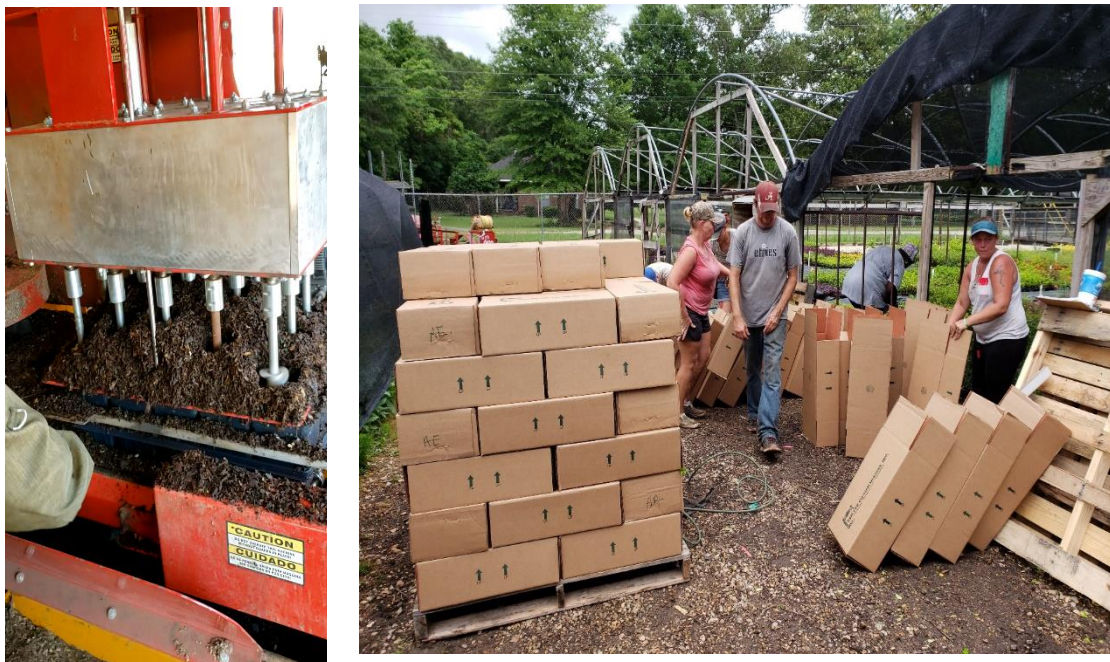
Figure 9. (left) Ellis Manufacturing built a 15-bit drill-head for our potting machine capable of producing jumbo quarts. (right) We can box and palletize the quarts to ship with our liners.
