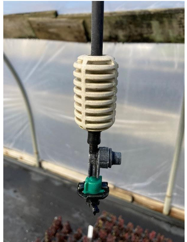
Figure 16. (Top, bottom left) Mini-Sprinklers are manufactured by Tavlit®. They are the 866 mini-compact sprinklers and can accommodate a variety of color-coded spinners which have different flow-rates. (Bottom right) An anti-drip device is included in the design to quickly discontinue the misting event.
