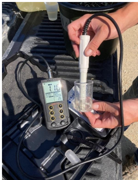
Figure 21. (left) Applying water to rooted cutting in order to provide leachate for analysis, and (right) measuring electrical conductivity and pH data of leachate to determine fertility level.
