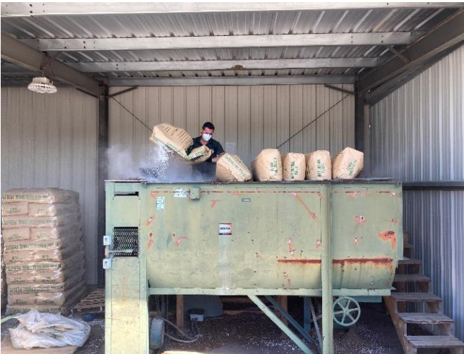
Figure 9. (left) Loading coarse perlite into 3.8 m 3 (5 yd 3 ) paddle mixer, and (right) loading bulk aged loblolly pine bark into the paddle mixer.
