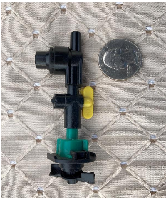
Figure 16. (Top, bottom left) Mini-Sprinklers are manufactured by Tavlit®. They are the 866 mini-compact sprinklers and can accommodate a variety of color-coded spinners which have different flow-rates. (Bottom right) An anti-drip device is included in the design to quickly discontinue the misting event.
