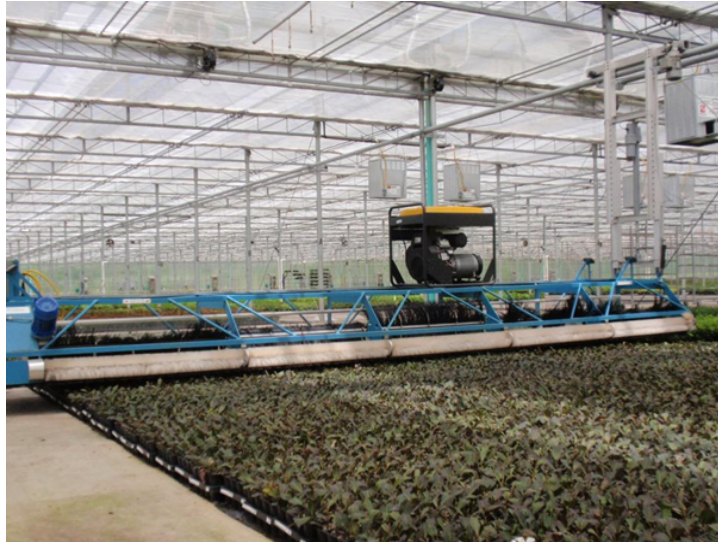
Figure 8. Completed 24-foot automatic trimming machine on rail system.
