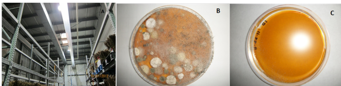
Figure 3. (A) Seasoning room with jet fan for distributing ozone. (B) A culture plate left open in the room for 15 h, without ozone. (C) The same test was done while ozone was actively being pumped through the air into the room.
