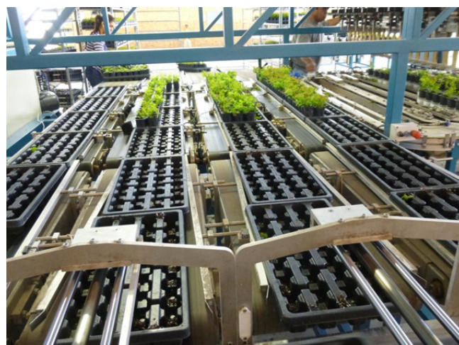
Figure 5. Tuinbouw Technisch Atelier (TTA) Plugsorter showing final grades.
